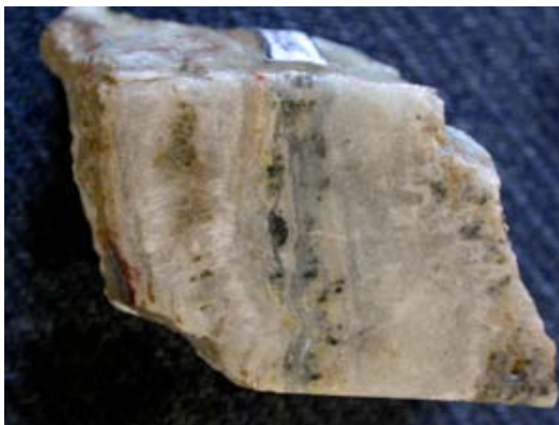
Figure 7.6 Cut Slab Showing Crustified Banding in Quartz-rich Vein Material
