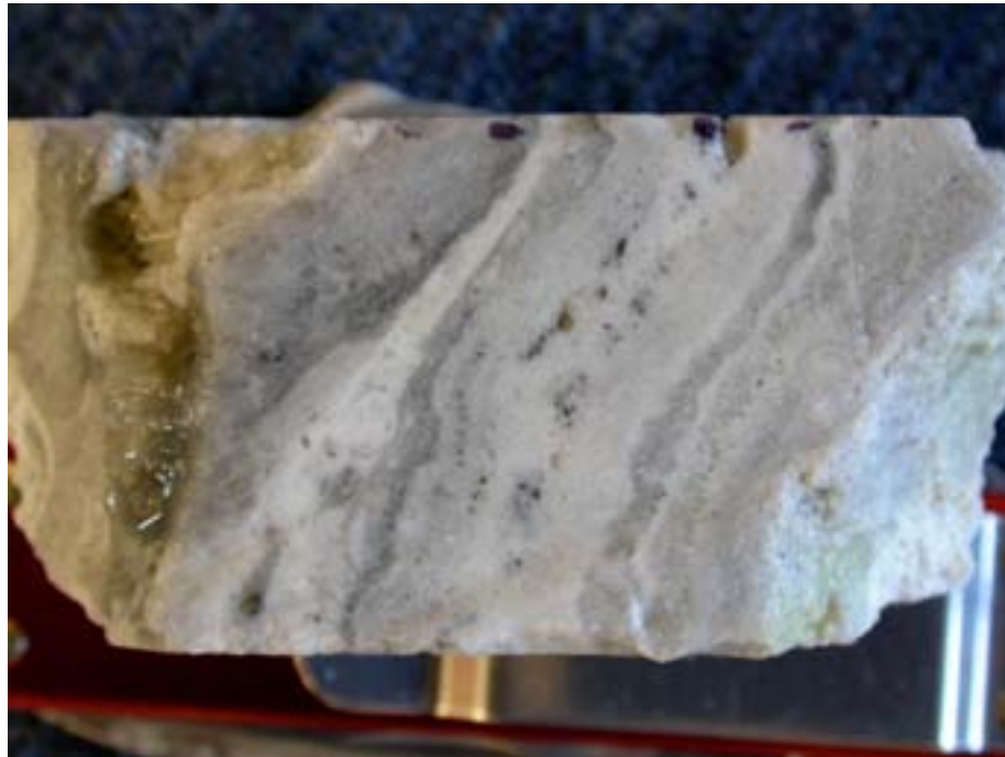
Figure 7.8 Core Sample Showing Crustified Vein Texture.
