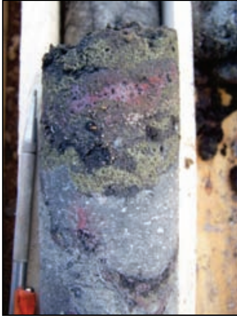
Figure 7-10 COSE Breccia (DDH-CSE-013D) exhibiting semi massive chalcopyrite and pyrargyrite- proustite, associated with pyrite, marcasite, and arsenopyrite
