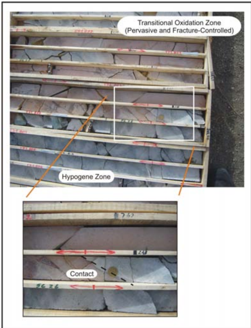
Figure 11.2 Example of Transitional Oxidized Zone with Transition to the Hypogene Zone, DDH CO-139-D
