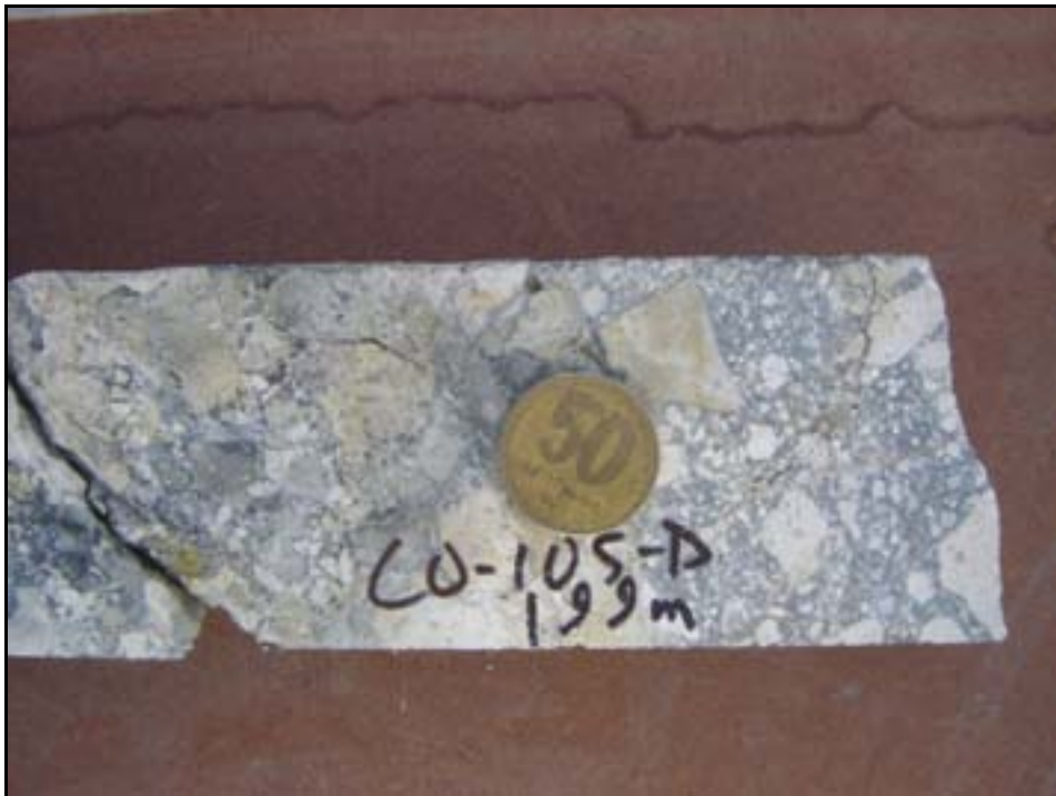
Figure 17.1 View of Mineralized Breccia, Cap Oeste Deposit (Interval Grades 9.22 g/t Au, 103 g/t Ag)
