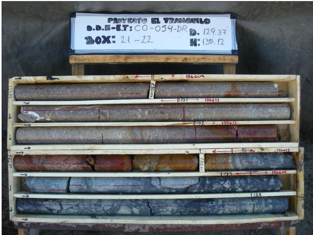
Figure 7-7 DDH Core from hole CO-054-D: Example of mineralized breccia in Zone 2b below silicified hematite rich oxidized fault contact
