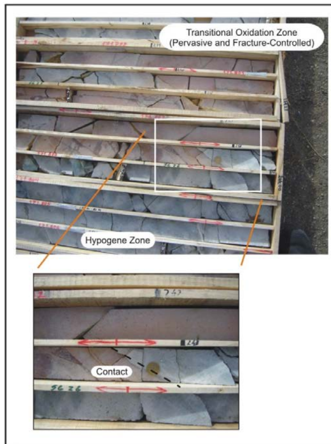
Figure 10-3 Example of Transitional Oxidized Zone with Transition to the Hypogene Zone, DDH CO-139-D
