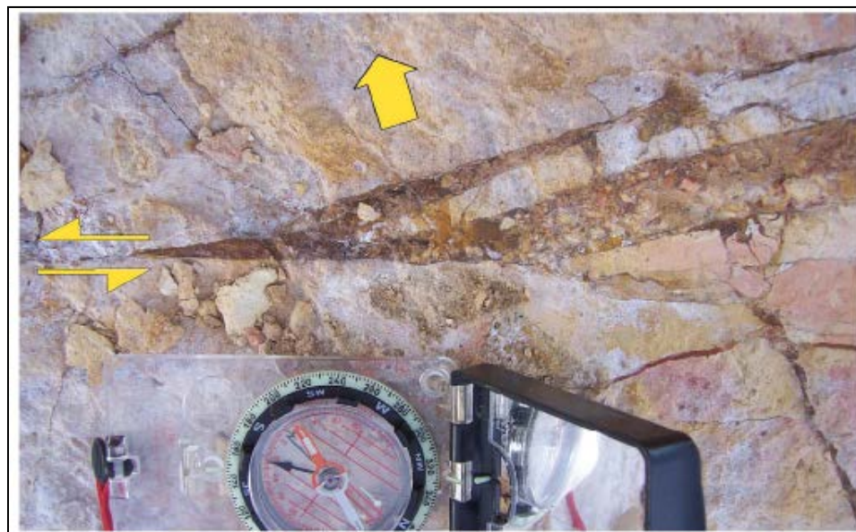
Figure 7-13 WNW trending tensional sulfide bearing veining splaying off a sinistral NW Fault (after Starling 2011)
