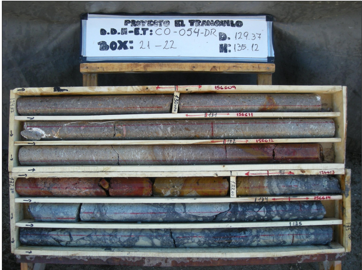
Figure 7-7 DDH Core from hole CO-054-D: Example of mineralized breccia in Zone 2b below silicified hematite rich oxidized fault contact (Source: PGSA 2011)
