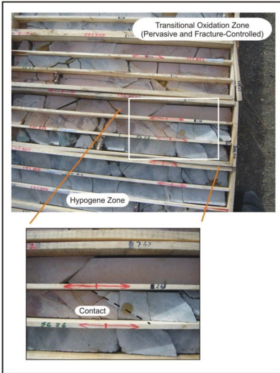
Figure 10-3 Example of Transitional Oxidized Zone with Transition to the Hypogene Zone
