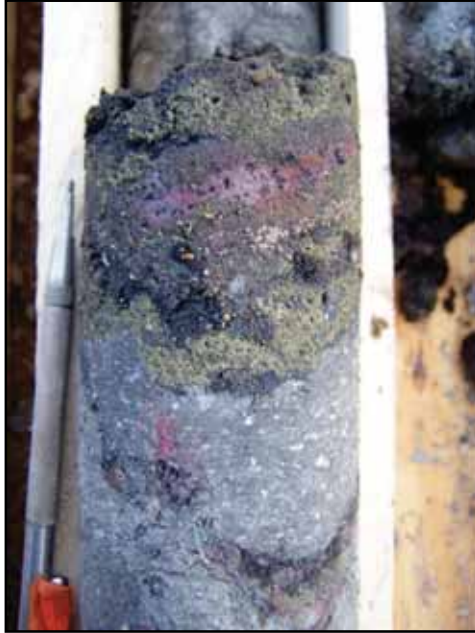
Photo 9-1 Cose Breccia (DDH-CSE-013D) exhibiting semi massive chalcopyrite and pyrrargyrite- proustite, associated with pyrite, marcasite, and arsenopyrite
