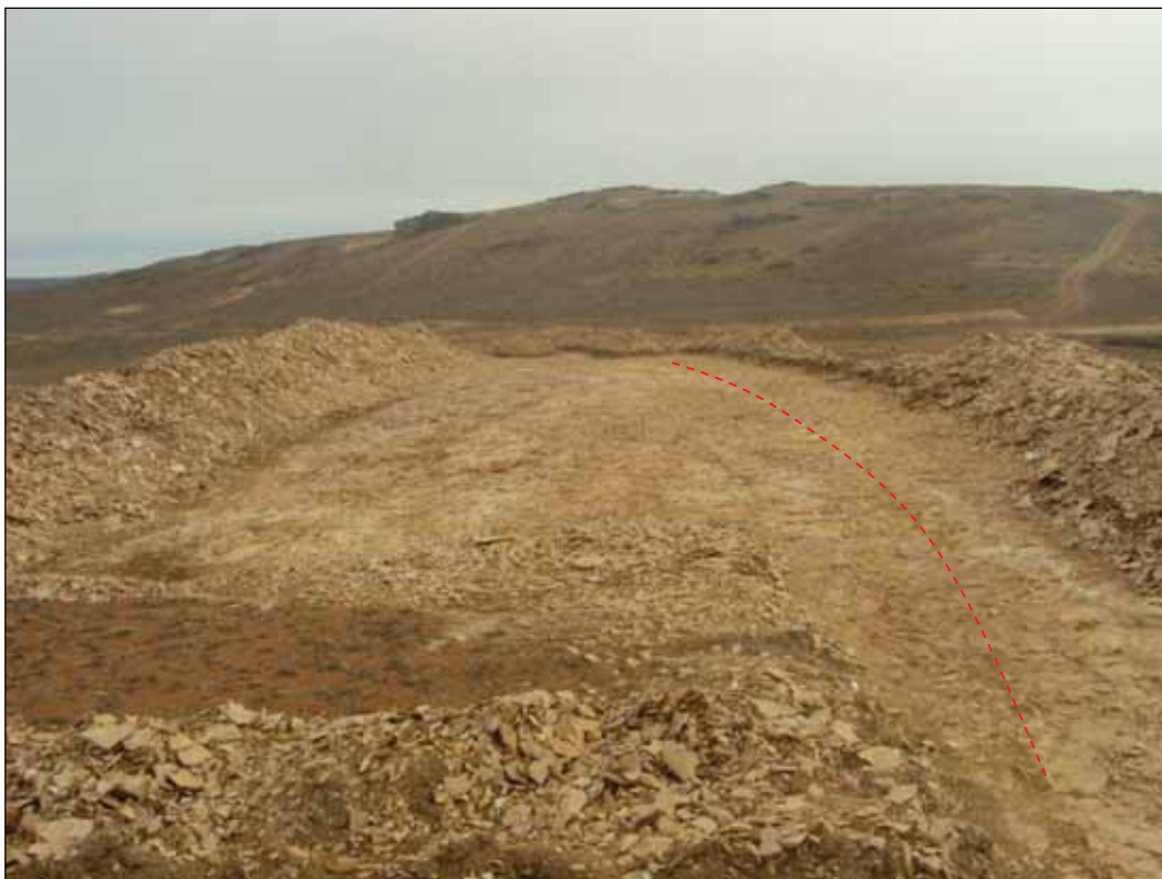
Photo 10-1 Excavation along the interpreted up-plunge expression of the COSE Breccia Shoot with annotated COSE Breccia Fault trace (red). Photo looks northwest.
